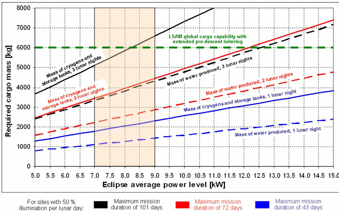
Figure 5: Cryogen storage requirements on LSAM for eclipse power generation at equatorial sites
