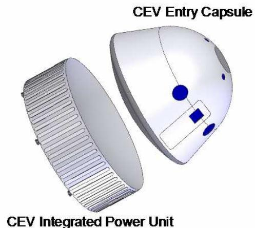
Fig. 6: Crew Exploration Vehicle (CEV) design with Entry Capsule and Integrated Power Unit modules.
